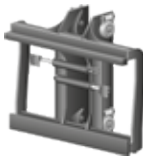
Carriage sideshift / fork positioning
