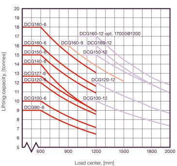
\* DCG100-6 to DCG180-6 models: Full lifting capacity up to 5,000mm lift height with duplex/duplex freelift/triplex masts and integrated sideshift/fork positioning carriage.
